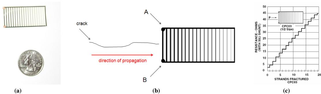
**FIGURE 2 (a) Photograph of crack propagation pattern with quarter for scale. (b) Measure resistance between points A and B. (c) Resistance can be correlated to number of broken sensor rungs (4).**
