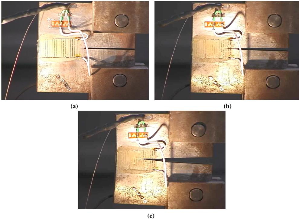
**FIGURE 6 (a) Test coupon with no crack. (b) Test coupon with six broken rungs. (c) Test coupon with eight broken rungs.**
