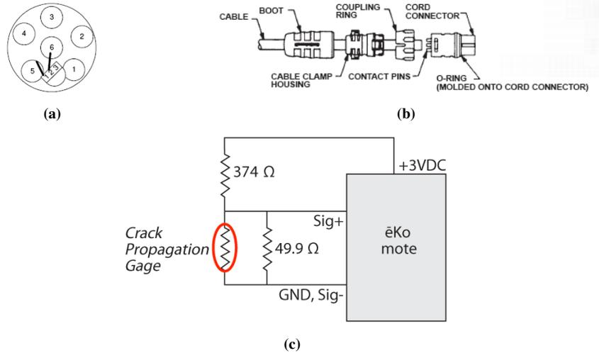
**FIGURE 3 (a) Schematic of EN3C6F connector housing with EEPROM mounted (5). (b) Water-tight cable assembly (7). (c) Diagram of sensor readout circuit, adapted from (4).**
