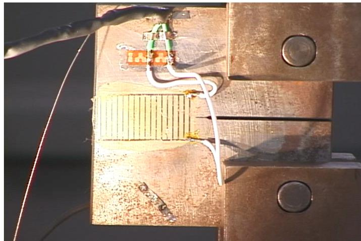
**FIGURE 4 Completed test coupon mounted in test apparatus.**
